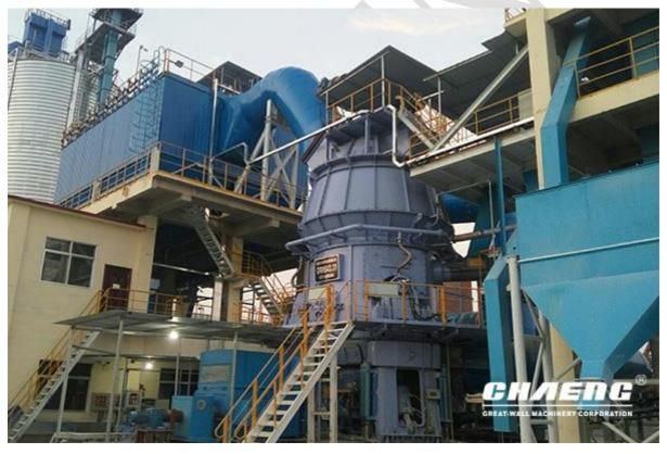
Great Wall Machinery can not only provide slag vertical mill equipment, but also undertake a **slag grinding production line** with an annual output of 200,000 to 1.5 million tons, and provide a complete set of EPC turnkey services. The supporting equipment includes belt feeder, vibrating screen, slag vertical mill, hot stove, dust collector and finished product warehouse, etc. Welcome to consult online or leave a message!
