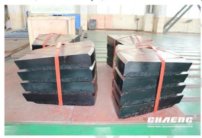
The performance of the liner will directly affect the performance of the ball mill. As the use time increases, the cylinder liner will inevitably be damaged during the grinding process. When the liner is 70% worn or there are 70mm long cracks on the surface, it is necessary to replace the liner in time.
